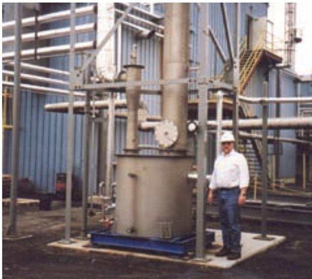
**Eductor Venturi/Packed Tower Combination Removes Particulate and Absorbs Alcohol Vapors** — A combined eductor/packed tower collector that removes solid particulate and absorbs alcohol has been successfully employed by this major specialty chemical producer.
