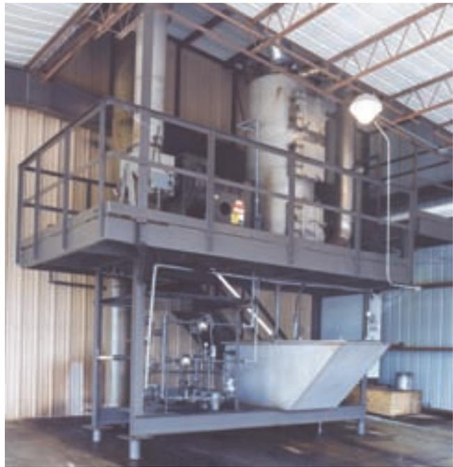
**Scrubber Cleans and Absorbs Acid Gases and Particulate From Medical Waste Incinerator** — An Impinjet® wet gas scrubber is used by this company to clean exhaust gases from its on-site medical waste incinerator.
