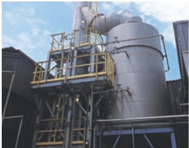
**Scrubber Collects SO<sub>2</sub> And Particulate At Reprocessor of Petroleum Catalysts** — An Impinjet® gas scrubber is used by this recycler of spent petroleum and chemical refining catalysts to clean flue gas from its ovens.
